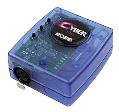
The Cyber Mini is the perfect product for small applications with less than 60 DMX channels. It offers a standalone memory with a maximum of 40 steps (60 channels) as well as 6 (4 + next/previous) ports for dry contacts triggering.
